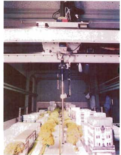
Figure 10 Endoscope and the street model
