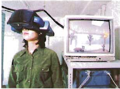
Figure 2 , A subject wearing the HMD is looking around the interior space of the scale model (The TV monitor shows the same visual image as the HMD)
