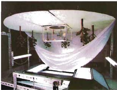
Figure 3 The simulation apparatus: a CCD color TV camera is inserted into the model space (The hemispherical cloth sheet is partially removed to show the inside)
